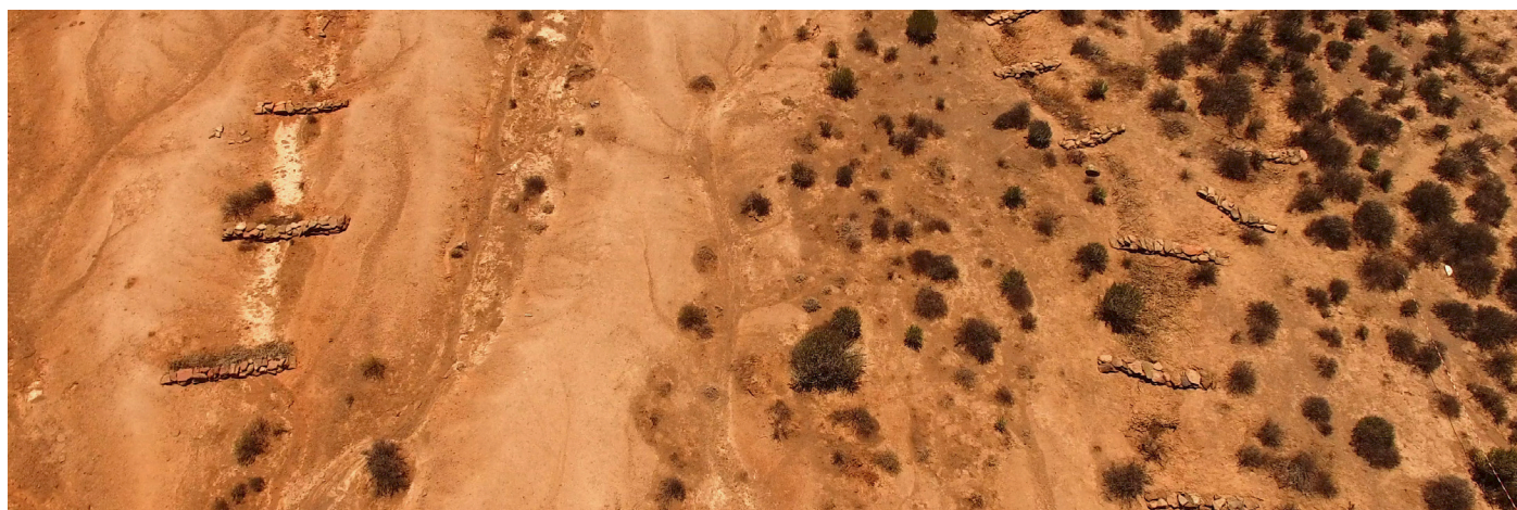
Figure 2 | Low cost erosion control structures tested for efficacy at capturing sediment and increasing water infiltration into gully eroded (top) and sheet eroded (bottom) paired sites within the BACIP experimental design.
